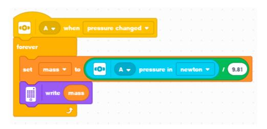
This program converts the force measured by the force sensor into mass based on this formula:
